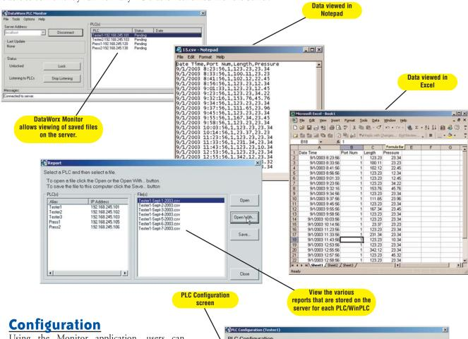
Using the Monitor application, users can configure the Server to log data to the Server's hard drive in a comma or tab delimited text file. Users can also include a date and time stamp in the file, and an alias for each data item sent. The alias can be used as the file's header.
